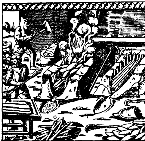
Fig 64 Liquefaction of crude copper (after AGRICOLA, de re Metallica )
