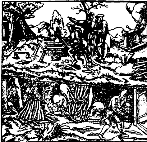
Fig. 14. Firesetting in a mine (after G. AGRICOLA, de Re Metallica )
