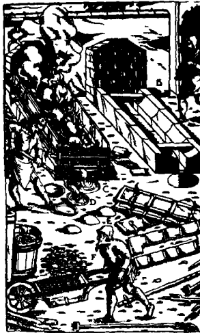
Fig. 43. Liquation of lead ores (after AGRICOLA, de re Metallica )
