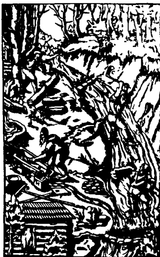
Fig 50 Collecting stream tin (after AGRICOLA, de re Metallica )
