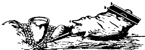
Fig 31 Primitive skin bellows of the Gypsy-smiths according to KOPERNICKI
