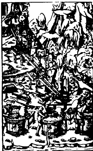
Fig. 51. Sluicing tin ore (after AGRICOLA, de re Metallica )
