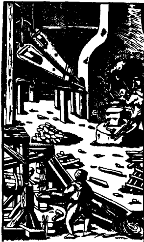
Fig. 88. Smithy with bellows, hammer, and quenching pit (after AGRICOLA, de re Metallica )
